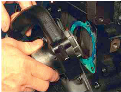
Figure 2.163 Water pump in water jacket
